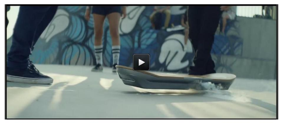
Main idea- Create a hoverboard that floats using permanent magnet and liquid nitrogen cooled super conductors
